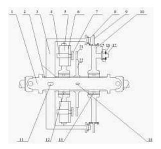
Fig. 1. structural schematic diagram of energy-saving self-excitation electromagnetic retarding device
