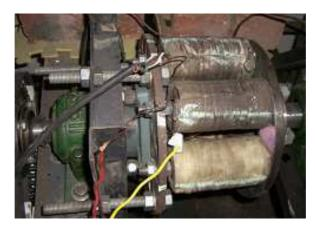
Fig. 3. energy-saving self-excitation electromagnetic retarding device
