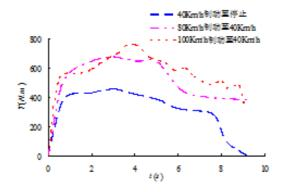
Fig. 4. variation curve of electromagnetic retarder torque with the braking time
